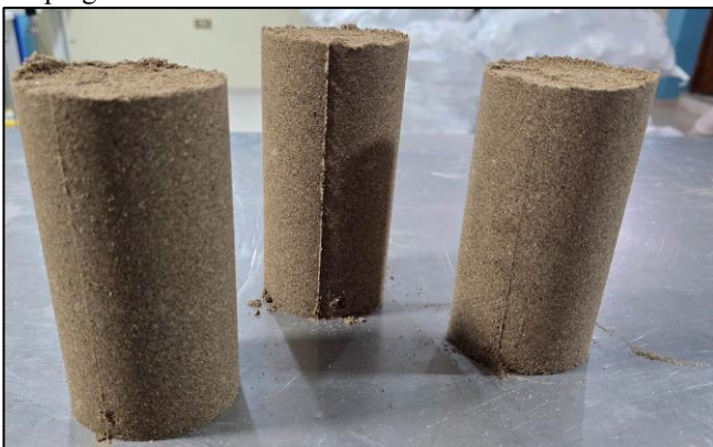
Fig. 17 Final specimens made by wet tamping
