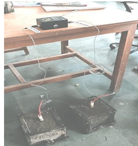
Fig. 3 CP-CMM with Concrete Cubes
